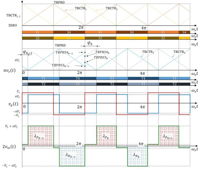
Figure 2: Theoretical waveforms by the original SPS modulation.
