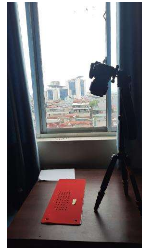
Figure 5: Setup for batch image capturing with camera, tripod and a batch of seed placed on a special paper to absorb hard lighting and facilitate background removal, seed segmentation later.
