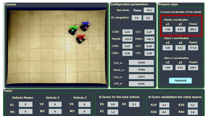
Figure 37: The results of the swarm robot moving in a triangle formation.
