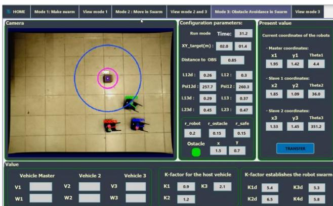
Figure 40: Results of the obstacle avoidance of the swarm robot.
