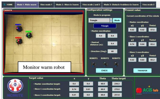
Figure 26: Interface for configuring and monitoring swarm robot.
