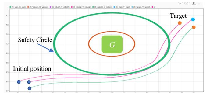
**Figure 25:** Obstacle avoidance of the swarm robot
