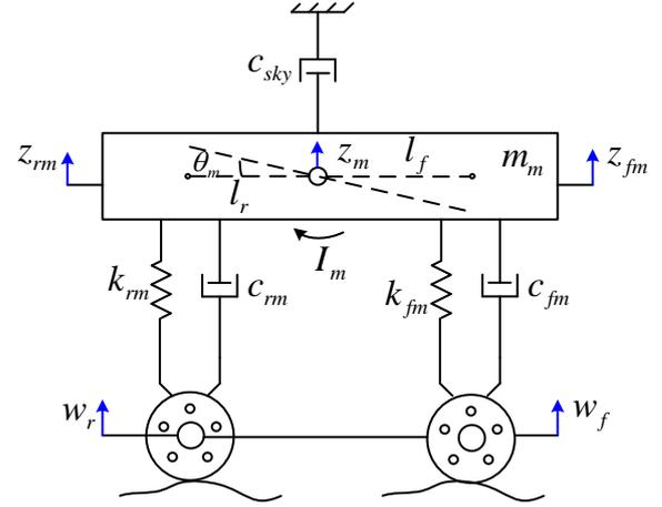
Figure 2: The proposed reference half-car model.
