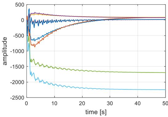
Figure 9: Convergence of the controller gains,  $K_r$ .
