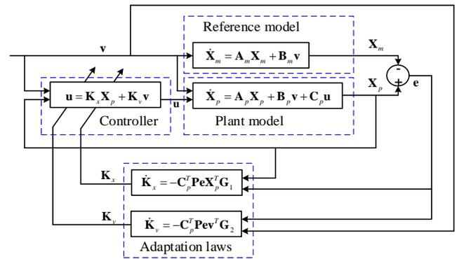
Figure 3: The MRAC scheme of active suspension system.
