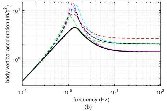
**Figure 4:** Frequency responses of vehicle body vertical acceleration with respect to the derivative of vertical displacement of a) front wheel, and b) rear wheel (solid line - reference system, dotted lines – passive system).
