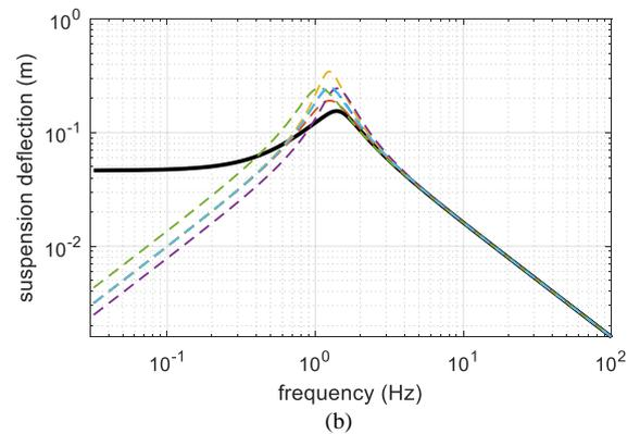
**Figure 5:** Frequency responses of suspension deflections at a) the front wheel and b) the rear wheel with respect to the derivative of vertical displacement of the front wheel and rear wheel, respectively, (solid line - reference system, dotted lines – passive system).
