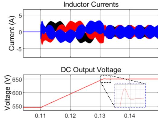
Figure 4: Matlab/Simulink simulation results of DC voltage, and inductor currents when the reference DC voltage ramp process is added
