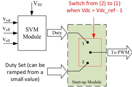
**Figure 9:** Constant duty ramp method block diagram
