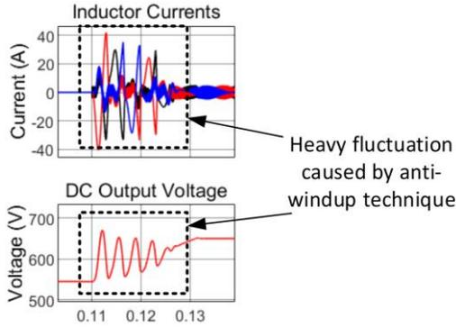
**Figure 5:** System response in the start-up procedure with RSPWM modulation method using Reference voltage ramp with anti-windup implementation.
