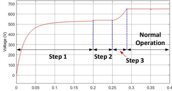
Figure 2: DC Output voltage during the start-up procedure
