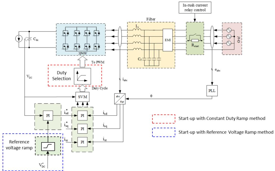
Figure 1: Control structure of the Three-Phase Four-Leg inverter
