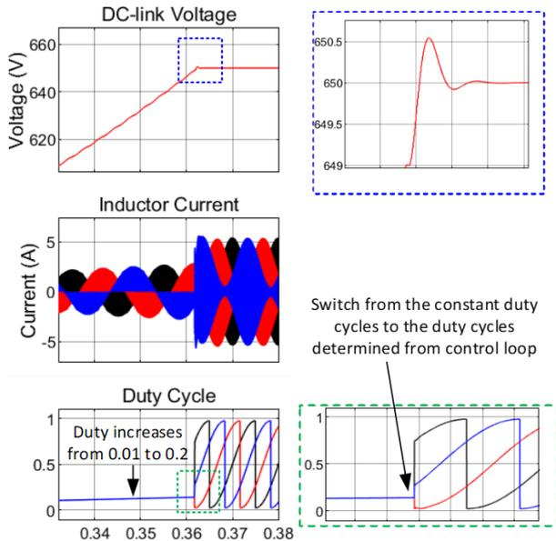
**Figure 10:** Simulation results of DC voltage, inductor currents, and duty cycles with the constant duty ramp method using the RSPWM modulation
