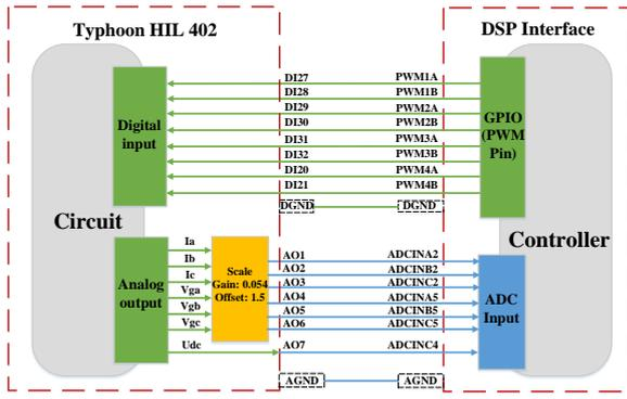
Figure 11: Pin configuration in the experiment setup
