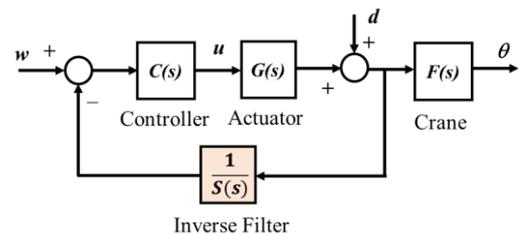
(c) Control structure with the inverse filter is in the feedback path of the trolley's position control loop
