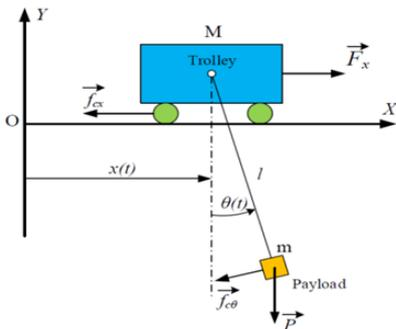
Figure 1: Overhead crane model
