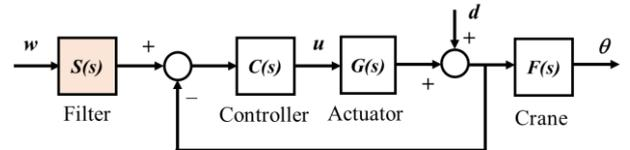
(a) Control structure with the filter is outside the position control loop
