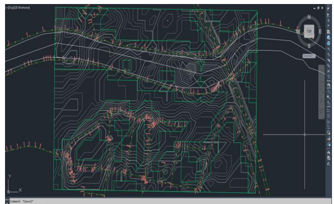
Figure 16. Proceed to create routes on Civil 3D.
