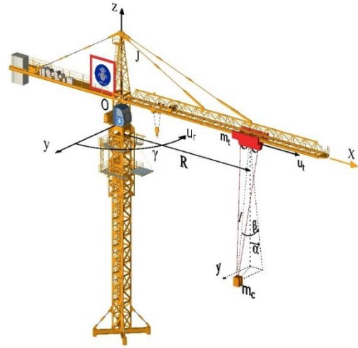
Figure 1. Tower crane model.
