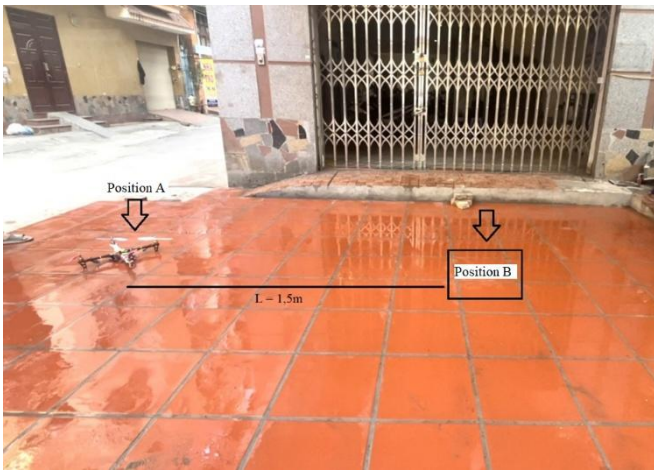
Figure 14: Test UAV take off at position A, fly to position B.
