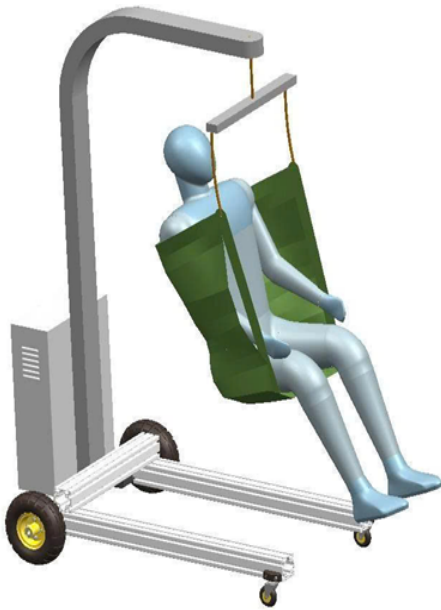
Figure 1: Mobile patient lifting and transferring system
