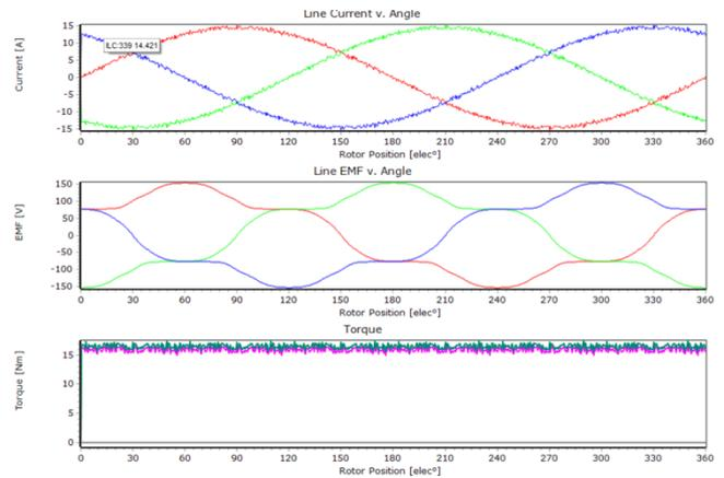
**Figure 5.** Phase Current, back EMF and torque of AFPM.
