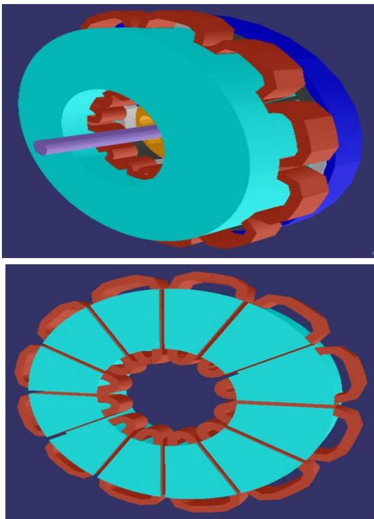
**Figure 4.** Detailed 3D structure of the proposed AFPM.
