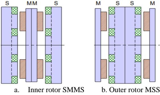
Figure 1. Variants of axial-flux permanent magnet motor
