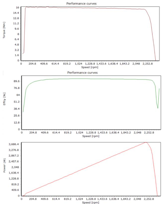
**Figure 6.** Distribution of the output torque (*top*), efficiency (*middle*) and power (*bottom*).
