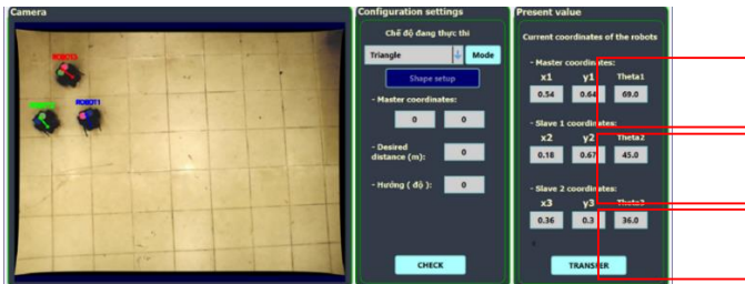
Figure 9: values of the position and direction of the mobile robot on the GUI
