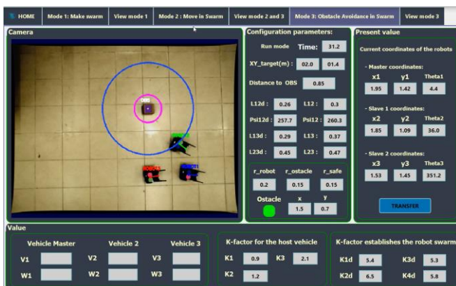
Figure 40: Results of the obstacle avoidance of the swarm robot.
